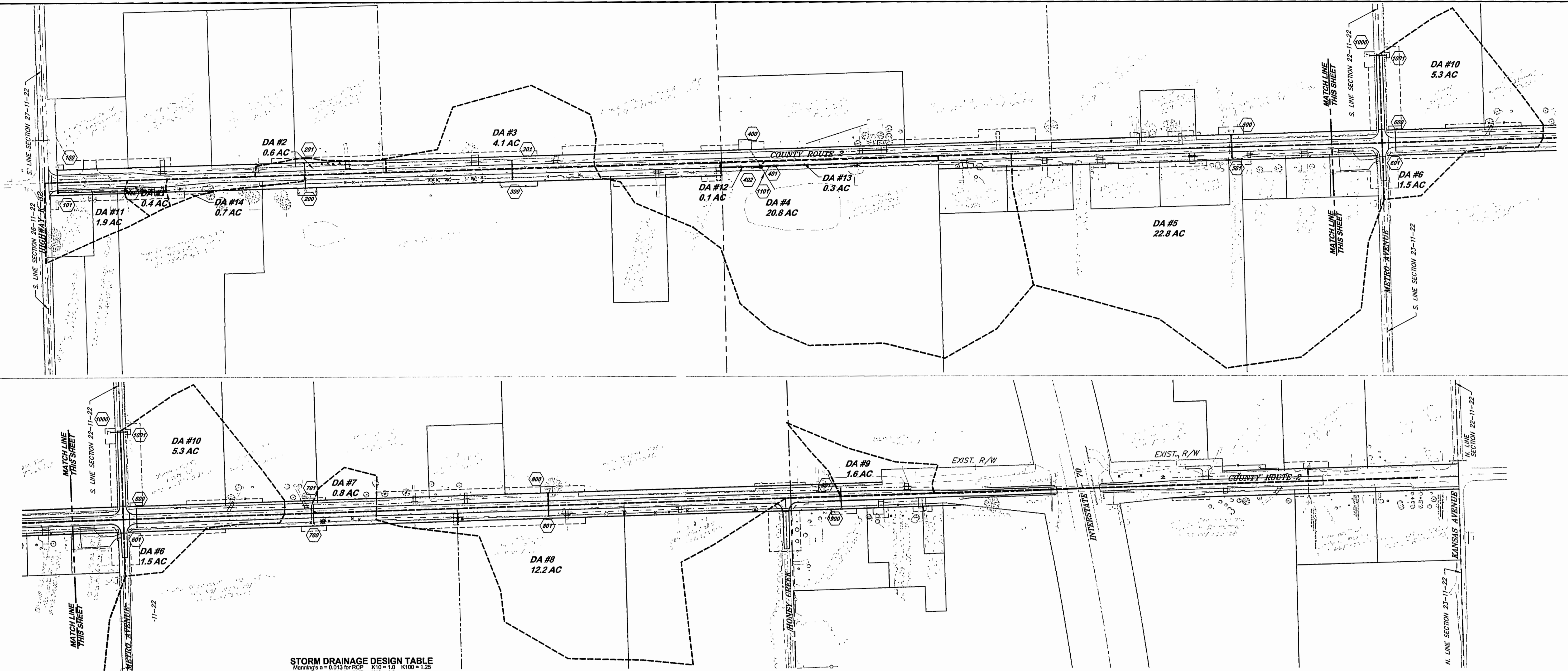
STORM DRAINAGE DESIGN TABLE Manning's n = 0.013 for RCP K10 = 1.0 K100 = 1.25 Manning's n = 0.024 for CMP K50 = 1.2
